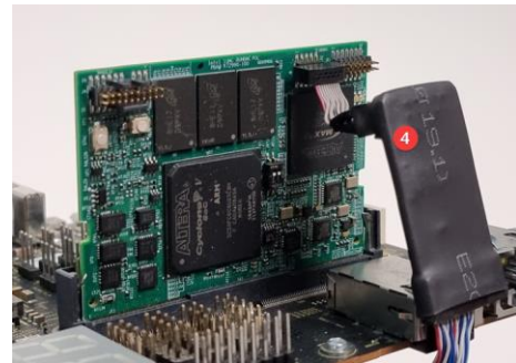
Picture 3, JTAG connection for FPGA programming
