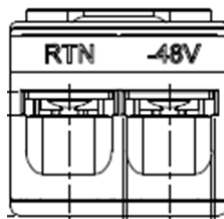
Figure 2-21 -48V Inlet connector (Telecom) pinout
