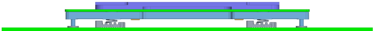
Figure 17 Side view (exploded) showing alignment pins being received by 1mm tall SMT nuts
